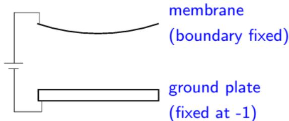
↔ control of voltage  $b(t)$  and/or design of dielectric properties  $a(x)$  to achieve prescribed displacement  $y_d(x, t)$ ;
